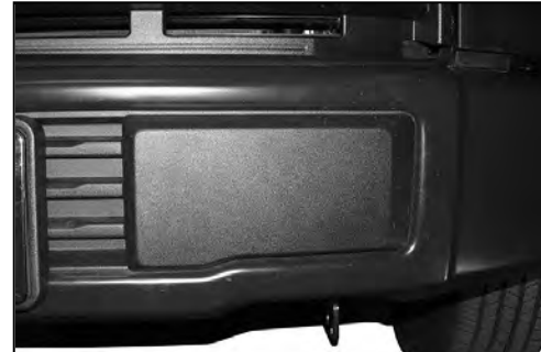
(Fig 5) Remove bumper pads to access splash guard hardware if necessary. 2015 F150 pictured
