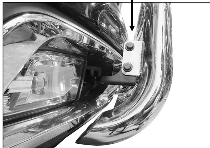
(Fig 13) Passenger/right side complete installation
