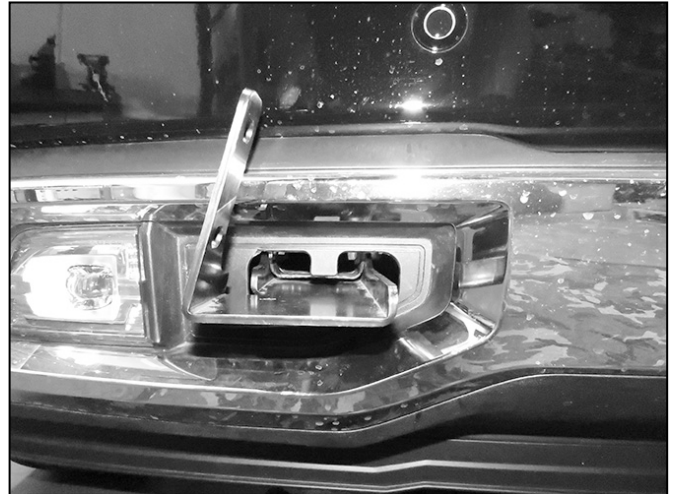
(Fig 11) Passenger/right side Bracket installed
