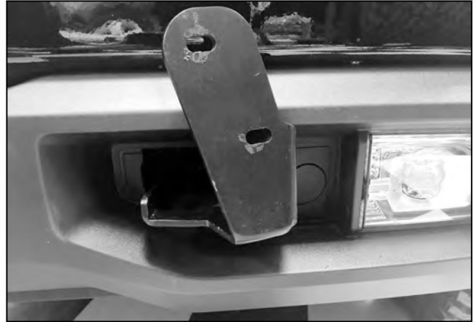
(Fig 11) Passenger/right side Bracket installed
