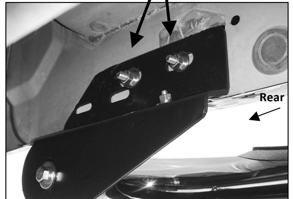
(Fig 4) Rear Mounting Bracket installation (except driver side Mounting Bracket on 97-98 3-door models)
