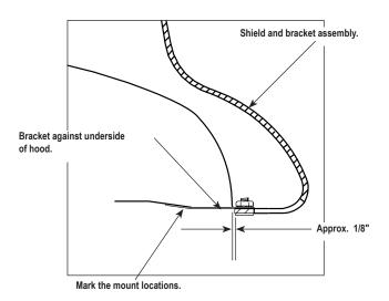
**3.** Remove shield from the vehicle and drill the marked mount locations. Use a 1/4" dia. drill bit.
