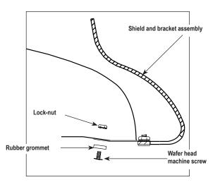
Caution: Carefully close hood after the shield has been installed. If the clearance is too tight between the shield and grill, hood and/ or grill adjustment may be required. Consult your owners manual or your dealer concerning hood grill adjustments.
