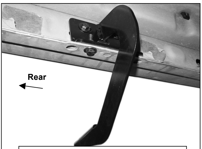
(Fig 10) Driver/left Rear Bracket installed
