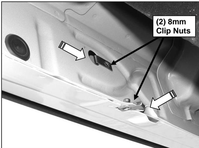
(Fig 3) Insert 8mm Clip Nut as required
