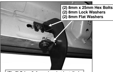
(Fig 7) Driver/left rear bracket installed
