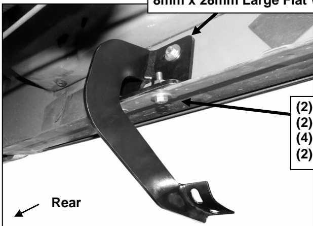
(Fig 3) Driver/left rear Mounting Bracket pictured
