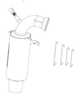
6. Re-install the factory temperature sensor. 2011-2012 models require use of the port extension.
