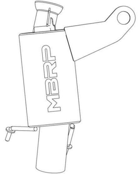
**NOTE:** To avoid exhaust leaks use a high heat silicone to seal all connections between the expansion chambers and the muffler. Monitor the exhaust for leaks during the first 200 miles after your installation and re-apply silicone where necessary. We suggest having your local snowmobile mechanic or performance shop install this product.
