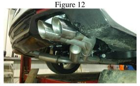
4. Install the OEM rear muffler hanger onto the **Driver-Side Tailpipe** as shown. Install a **3**" **Clamp** onto the inlet. **Refer to Figure 9.**
