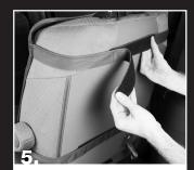
Attach hook & loop straps behind seat back.
