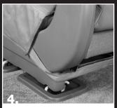
Attach hook & loop strap behind the lower part of the seat back.
