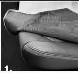
Unroll cover. Place seat bottom portion grippy side down and fold seat back portion over onto bottom portion. Ensure the half with straps is on top.
