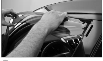
Bow the deflector outward and insert the end into the S-Clip installed in step 2.
