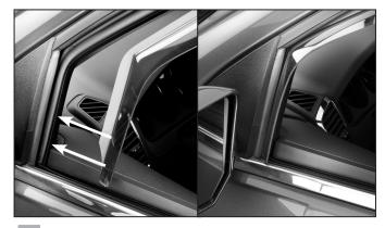
Insert the front of the part as shown; ensure edge rests on top of the outer window sill.
