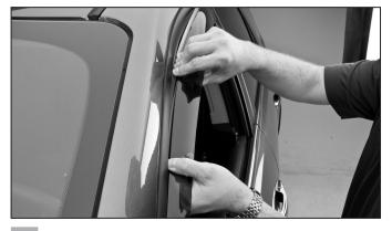
Starting from the front of the part, begin tucking the flange into the window channel.
