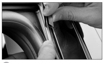
Push back the weather stripping on the rear end of the window and insert the S-Clip as shown.
