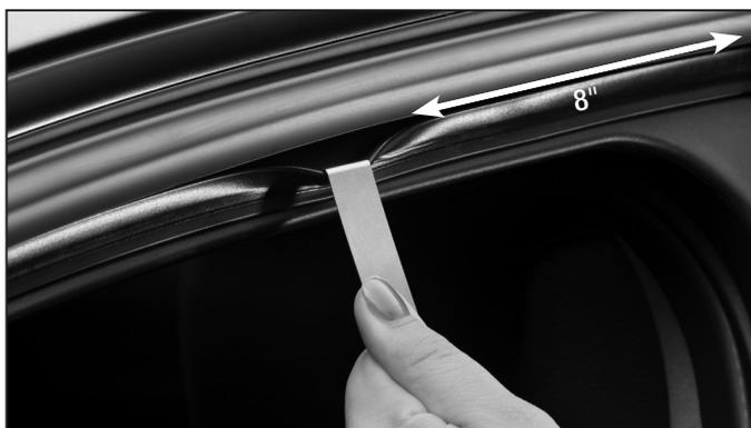
**1** Make sure that the window is clean and dry. Then pull down the weather stripping in the first position, which is approximately 8" from the rear of the deflector.
