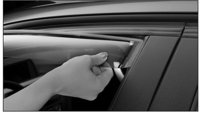
**6** Bow the deflector outward to insert the rear flange into the window channel. Making sure the window gasket is not folded over.
