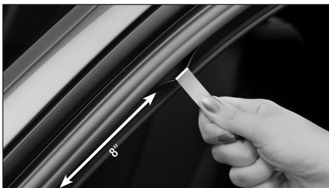
**3** Pull down the weather stripping in the second position, which is approximately 8" from the front mirror.
