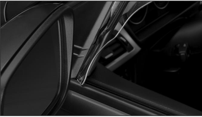
**5** Insert the front of the deflector as shown. Ensure that the edge rests on the top of the outer window sill.
