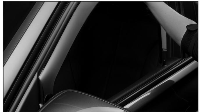
**8** Inspect the deflector to ensure that it is fully inserted into the window channel. Slowly and carefully, close your window fully and press firmly against weather strip from front to rear without engaging auto-up feature.
