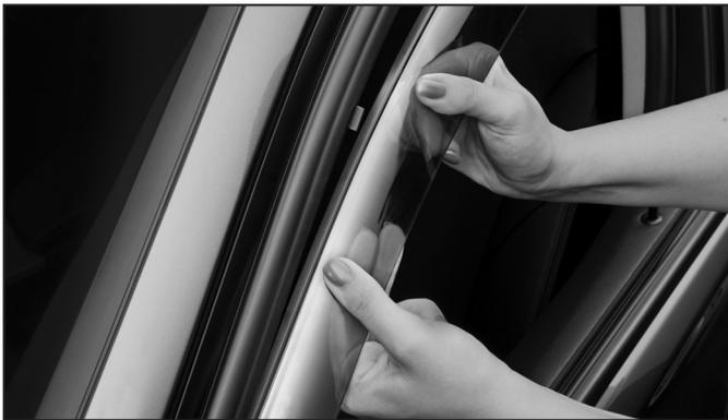
**7** Starting with the front of the deflector, begin tucking the flange into the window channel while pressing inward against the channel clips. Be sure to tuck the flange between weather stripping and the channel clip.
