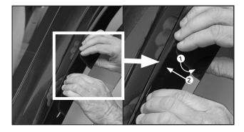
Pull down and tuck in working from front to back.
