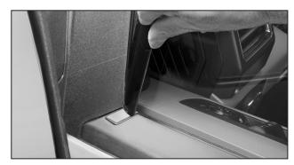
Lower the front of the deflector onto the weatherstrip clip as shown.
