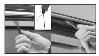
Run the seating tool between deflector and window seal to set the deflector. Repeat steps 1-9 on the passenger side.
