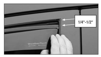
Insert the rear edge leaving a gap at the top.
