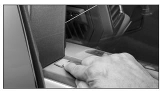
Place the weatherstrip clip onto the window gasket material: postion as far forward as possible.
