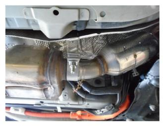
**Step 6.** Finish installation by tightening clamp and fasteners to torque specifications.
