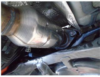
**Step 5.** Install the supplied clamp onto new MagnaFlow converter end and install over cut pipe on vehicle. Bolt converter flange into place using the OF fasteners.
