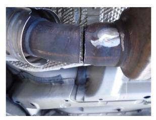
**Step 4.** Cut pipe at marked location. Loosen fasteners from inlet flange and remove converter. Clean and deburr cut pipe remaining on vehicle. (Retain fasteners to be used on installation of new MagnaFlow part)
