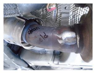
**Step 2.** Once heatshield is removed clean up weld burr.
