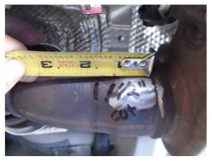
**Step 3.** Measure 1 1/2" (38cm) from edge of weld (on heat exchanger) and mark.
