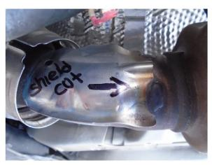
**Step 1.** Begin by Grinding (to remove) the weld attacing the heat shield to the converter pipe and remove the heatshield.
