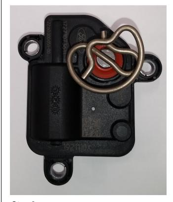
**Step 2**. If the spring were to detach, reinstall in orientation seen above.
