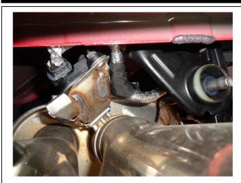
**Step 1.** Unplug the electrical connection on the Exhaust Valve Control Motors (Qty 2) located on the OEM exhaust assembly, also disconnect wire harness mounting plug.
