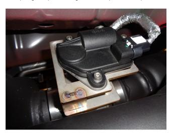
**Step 4**. Valve orientation should be placed with the electrical plug facing the rear of the vehicle. Rotate valve to be free of any interference like the body, exhaust system or hangers that can damage the valve. Once a final position has been chosen for the new valve system, evenly tighten all clamps from front to rear. Re-connect the wiring harness plug to the Valve motors and wire mounting bracket. Inspect all fasteners after 25-50 miles of operation and re-tighten if necessary.
