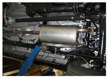
**Step 1.** Begin removing the OEM exhaust by unbolting the spring loaded coupling flange at the outlet of the OEM Y-Pipe that attaches to the muffler inlet with a 14mm socket.
