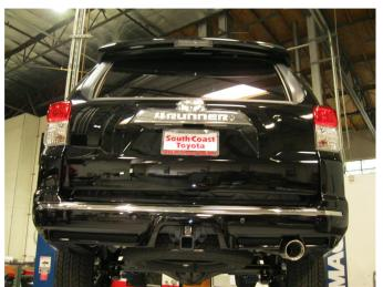
**Step 5.** Once a final position has been chosen for the new system, evenly tighten all fasteners from front to rear using the torque specifications on page one of this document. Inspect all fasteners after 25-50 miles of operation and retighten if necessary.
