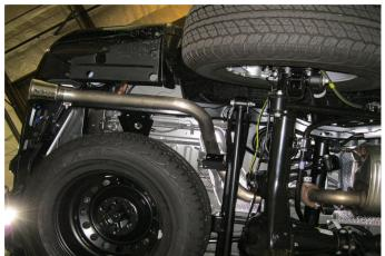
**Step 2.** Next unbolt the outlet of the OEM muffler at the inlet of the tail pipe assembly. Remove the welded hangers from the rubber insulators using a pry bar. do not discard or damage the insulators as they will be needed to install your new system. The OEM system may now be removed.
