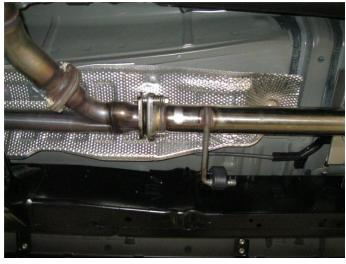
**Step 3.** You are now ready to install your new MAGNAFLOW system. Attach the the Inlet Pipe Assembly to the OEM Y-Pipe outlet using the existing hardware. Engage the welded hanger to the OEM rubber insulator. Leave all clamps and hardware loose for final adjustment of the complete system.
