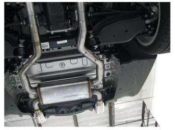
**Step 2.** Begin installation of the new system by fastening the Inlet Pipe Assemblies to the pipes you have just cut using the supplied 2.25" clamps. Locate the welded hangers to the rubber insulators. (Leave all clamps and fasteners loose for final adjustment of the complete system.)
