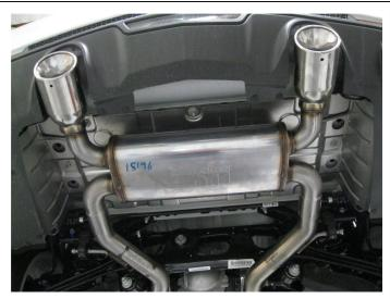
**Step 3.** Next Install the Muffler Tail Pipe Assembly to the outlets of the Inlet Pipe Assemblies using the supplied 2.50" clamps. Insert hangers into rubber insulators.
