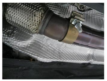
**Step 3.** Begin installing your new system by first attaching the OEM hanger assemblies you removed to the new system. At this stage you may also replace the underbody cross-mamber. Next, looseley secure the Inlet Pipe Assembly to the OEM flex pipe outlet using the supplied clamp.
