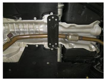
**Step 1.** Before removing the OEM exhaust system you will need to first remove the underbody cross-member using a #50 male TORX socket.
