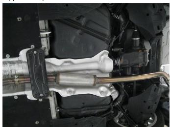
**Step 4.** Loosely install the Resonator and Muffler Tail Pipe Assemblies using the supplied.2.50" clamps. Reattach the OEM hanger assemblies.
