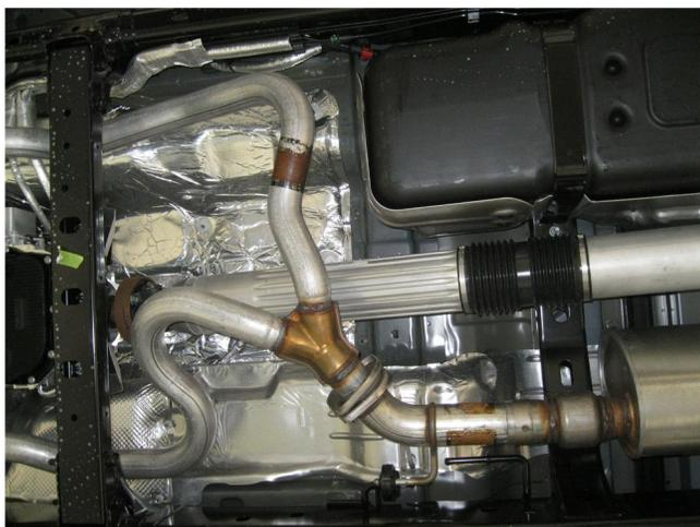
**Step 1.** To remove the OEM exhaust system, you will first need to unbolt the muffler assembly from the Y-Pipe assembly.
