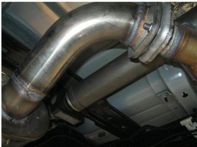
**Step 3.** You are now ready to install your new MAGNAFLOW exhaust system. Begin by bolting the inlet flange of the Muffler Assembly to the Y-Pipe assembly using the OEM hardware. Engage both welded hangers to the rubber isolators.
