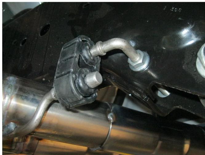
**Step 4.** To support the Tail Pipe Assembly you will need to locate the supplied threaded hanger through two existing holes in the vehicles sub frame. Secure with the supplied hardware as shown.
