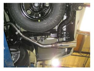
**Step 4.** Complete the installation by fastening the Driver and Passenger side Tailpipe Assemblies to the Extension Pipe Assemblies with the supplied 2.50" clamps and fit the hangers into the insulators.
