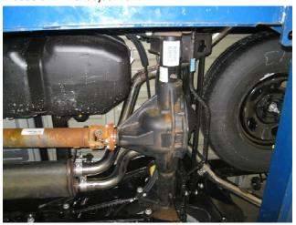
**Step 3.** Next Install the Driver and Passenger side Extension Pipe Assemblies using the supplied 2.50" clamps and fitting the hangers into the rubber insulators.
