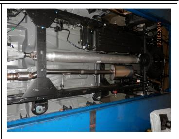
**Step 3.** Only Crew Cab with 78.8in. Bed vehicles will require the 12.5" Extension Pipe to be fitted between the Inlet Pipe Assembly and the Muffler Assembly. Loosely attach the Muffler Assembly using the supplied clamps. Engage all welded hangers to the rubber insulators.
