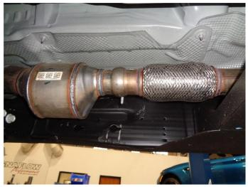
**Step 1.** To remove the OEM exhaust loosen the clamp at the ball flare junction attachiong the inlet pipe to the catalytic converter outlet. Working front to rear disengage all welded hangers from the rubber insulators. Be sure to retain all mounting hardware as it will be needed to install your new MAGNAFLOW system.
