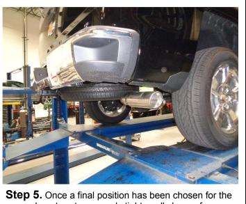
**Step 5.** Once a final position has been chosen for the new exhaust system, evenly tighten all clamps from front to rear using the torque specifications on page one of the instructions. Inspect all fasteners after 25-50 miles of operation and re-tighten if necessary.
