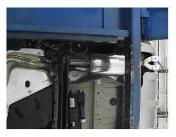
**Step 8.** Working front to rear install the remaining parts in the same fashion as the Inlet Extension Pipe, fitting hangers into rubber insulators and keeping clamps loose.
