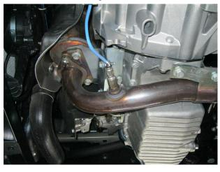
**Step 3.** Remove the O2 sensor (Unplug the wire connector the prevent damge to the wires)
