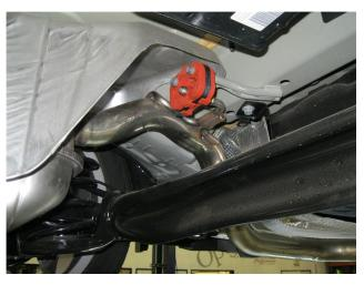
**Step 4.** Disengage the the exhaust hangers from the rubber insulators (Save the insulators as they will be re-used on the new system)
