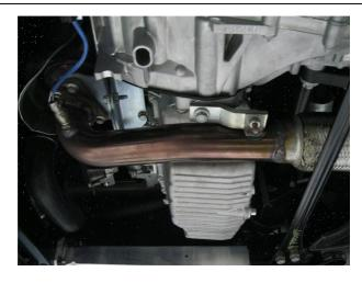
**Step 6.** Begin installation of your new MAGNAFLOW exhaust system by attaching the Inlet Pipe Assembly using the OEM nuts at the flange and the OEM bolt and supplied M8 nut at the transmission mount. Insert hangers into OEM rubber insulators and re-install the cross brace and o2 sensor.
