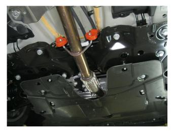
**Step 1.** Start by removing the engine shield at the front of the vehicle. Underneath this shield is a cross brace that must also be removed.
