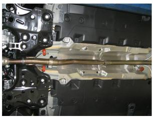
**Step 7.** Next, install the Front Extension Pipe using the supplied 2.25" clamp (keep clamps loose until final adjustment of system).
