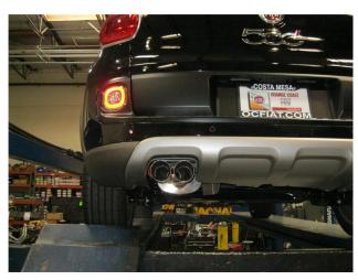
**Step 9.** Once a final position has been chosen for the new exhaust system, evenly tighten all clamps from front to rear using the torque specifications on page one of the instructions. Finish by re-installing the engine shield. Inspect all fasteners after 25-50 miles of operation and re-tighten if necessary.
