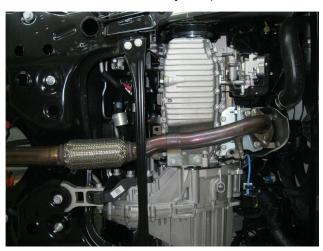
**Step 5.** Un-fasten the exhaust from the bracket attaching it to the transmission. Un-fasten the nuts attaching the flange at the bottom of the exhaust manifold and remove exhaust.
