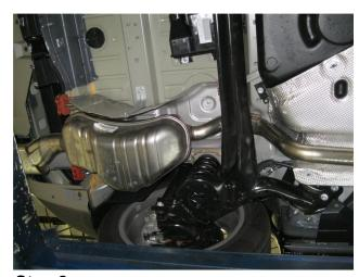
**Step 2.** Using a Sawzall (or other cutting device) cut the OEM exhaust just in front of the rear muffler. This step is critical as the exhaust cannot be removed without cutting.
