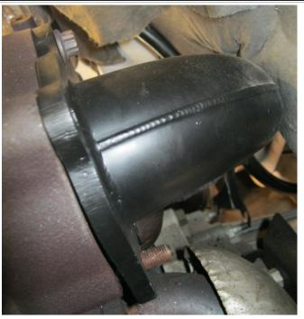
Step 3. Install your new downpipe by first attaching the Inlet flange to the turbo. Using the existing OEM harware hand tighten the new MagnaFlow downpipe to the Turbo. Then install the clamp onto the outlet and connect to the exhaust system
