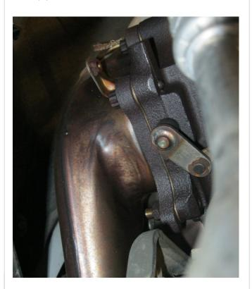
Step 2. After all fasteners have been removed, remove the OEM Downpipe.
