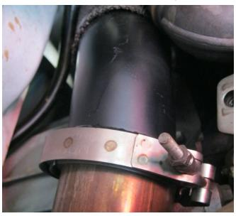
Step 4. Once a final position has been chosen for the new downpipe, evenly tighten all bolts and clamps from front to rear using the torque specifications on page one of the instructions. Inspect all fasteners after 25-50 miles of operation and re-tighten if necessary.
