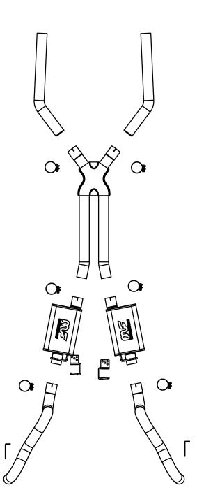
**Note:** This system is designed to work with OEM-style exhaust manifolds, or tubular headers. Due to the various applications possible, some modification and welding is required for a proper fit and finish.
