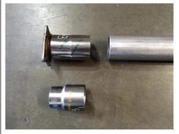
**Step 2.** Before installing your new system select the correct inlet adapter for your vehicles year. The larger adapter with the flange attached covers '01 - '05, the slip adapter covers '06 - '07. Attach the appropriate adapter by either bolting it to he vehicle outlet using the OEM fasteners or inserting the adapter into the slip clamp and loosely securing.
