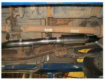
Step 5. Install the Muffler Assembly, Over Axle Pipe and Tail Pipe Assembly in a similar fashion to the Extension Pipe Assembly using the supplied clamps. Engage all welded hangers to the rubber insulators.
