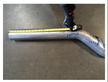
**Step 3.** The inlet end of the Mid Pipe Assembly may need to be trimmed depending on the year and cab configuration of your vehicle.
