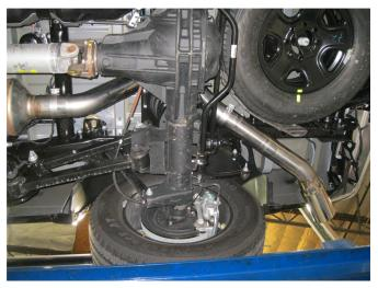
**Step 6.** Next Install the Tail Pipe Assembly in a similar fashion using the supplied 4.00" clamps and by fitting the welded hangers into the rubber insulators.
