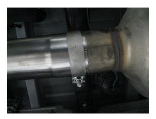
**Step 1.** Begin removal of the OEM system by unclamping the OEM Extension Pipe and muffler from the junction behind the DPF. You can then disengage the welded hangers from the rubber insulators, working rearward finish removing the system. Do not damage or discard the rubber insulators or sensor bracket and fastener, as they will be reused to mount the new system.
