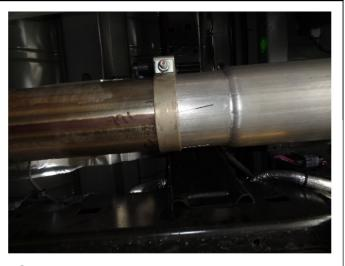
**Step 2.** Your vehicle configuration will determine which inlet pipe is used, see the table below. Begin installation of the MagnaFlow system by attaching the appropriate Inlet Pipe to the outlet of the DPF using the supplied 4.50" clamp.
