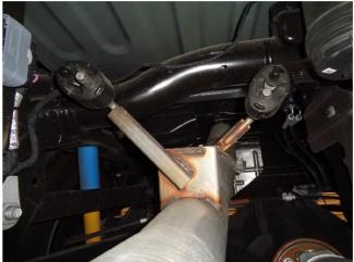
**Step 1.** Remove the OE system by unclamping the OE Extension and Tail Pipes from the junction behind the DPF. Disengage the welded hangers from the rubber insulators, working rearward finish removing the system. Do not damage or discard the rubber insulators as they will be reused to mount the new system.
