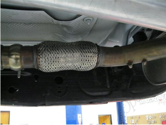
**Step 1.** To Remove the OEM system, you will need to cut the exhaust pipe behind the muffler before it goes over the axle. Next disengage the welded hangers from the rubber insulators and remove the tail pipe. Unclamp the muffler inlet from the catalytic converter at the clamp junction. Do not damage or discard the OEM fasteners or rubber isolators, as they will be reused to mount your new MAGNAFLOW system.
