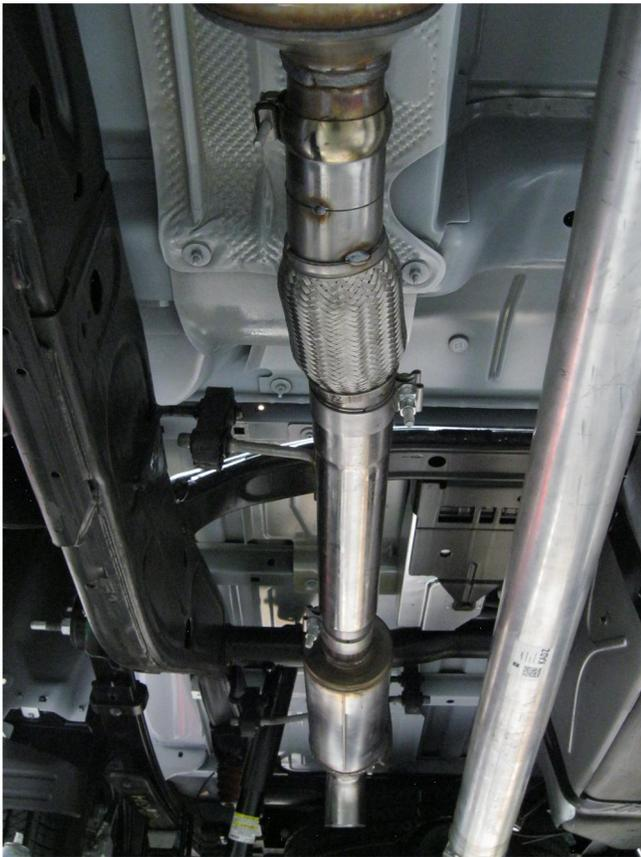
**Step 2.** Install the new Inlet Pipe Assembly at the ball flare using the OEM fastener. Install the Mid Pipe Assembly by slipping the inlet over the outlet of the Inlet Pipe Assembly. Then loosely secure using the supplied 3.00" clamp.
