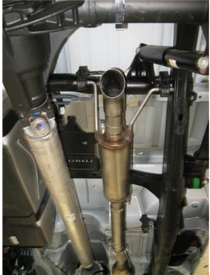
**Step 3.** Install the Muffler Assembly and tail pipe following the same procedure using the supplied 2.50" clamps and by fitting the welded hangers into the OEM rubber isolators. Leave all clamps and fasteners loose for final adjustment of the complete system.
