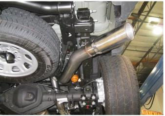
**Step 3.** Next Install the Tail Pipe Assembly in a similar fashion using the supplied 4.00" clamps and by fitting the welded hangers into the rubber insulators.
