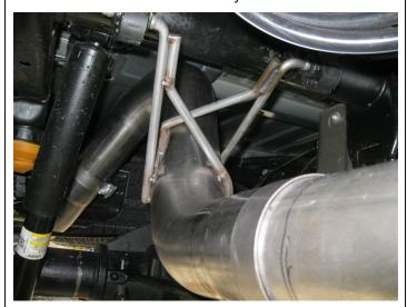
**Step 2.** Begin installation of the Magnaflow system by clamping the Inlet Pipe to the newly cut outlet of the DPF using a supplied 4.00" clamp and fitting the hangers in the rubber insulators (leave all clamps loose for final adjustment of the complete system). If your vehicle has an O2 sensor re-install at this time. If not, install the provided sensor boss plug.
