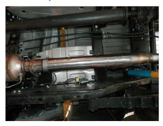
**Step 2.** Begin installation of the Magnaflow system by locating the indexing notch to the OEM peg then loosely clamping the Inlet Pipe to the outlet of the DPF using a supplied 4.00" clamp. Install the Over Axle Pipe in a similar fashion
