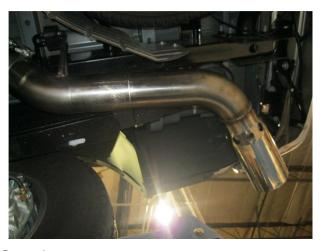
**Step 3.** Finish by installing the Taipipe Assembly to the inlet pipe using a supplied 4.00" clamp and fitting the welded hanger into the rubber insulator.
