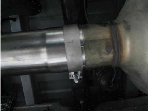
**Step 1.** Begin removal of the OEM system by unclamping the OEM Extension Pipe and muffler from the junction behind the DPF. You can then disengage the welded hangers from the rubber insulators, working rearward finish removing the system. Do not damage or discard the rubber insulators or sensor bracket and fastener, as they will be reused to mount the new system.
