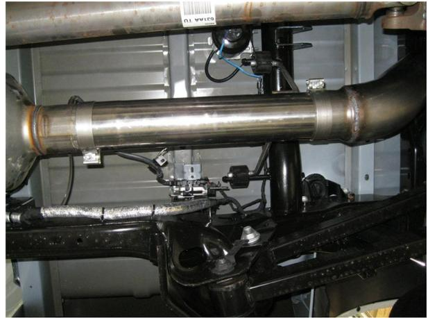
**Step 3.** The longer Inlet Pipe Extension will be needed for Long Bed applications only.
