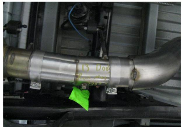
**Step 5.** The shorter Inlet Pipe Extension will be needed for all Mega Cab applications.
