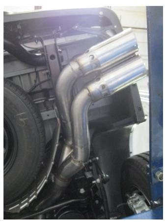
**Step 6.** Next install the Tail Pipe Assembly using the supplied 4.00" clamp and fit the welded hanger to the rubber insulator.
