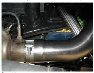
**Step 2.** Begin by attaching either the Inlet Pipe options or the Over Axle Pipe to the DPF outlet using the supplied clamp. Fit hangers into rubber insualtors on Mega Cab and Long Bed versions. Leave all clamps loose until final adjustment.
