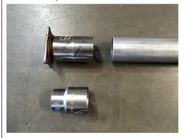
**Step 2.** Before installing your new system select the correct inlet adapter for your vehicles year. The larger adapter with the flange attached covers '01 - '05, the slip adapter covers '06 - '07.5. Attach the appropriate adapter by either bolting it to he vehicle outlet using the OEM fasteners or inserting the adapter into the slip clamp and loosely securing.
