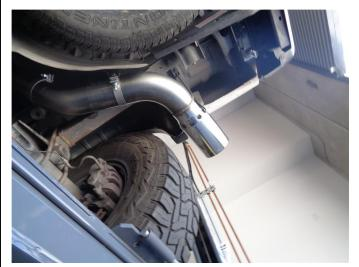
**Step 5.** Loosely slip the Hanger Clamp Assembly over the Tail Pipe Assembly. Loosely install the Tail Pipe Assembly using the supplied clamp. Engage the welded hanger to the rubber insulator.
