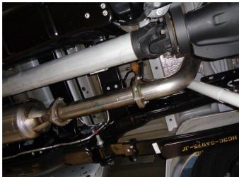
**Step 1.** To remove the OEM exhaust remove the O2 sensor from the over axle pipe (6.7L only). Unbolt the extension pipe assembly from from the DPF outlet flange (6.7L) or loosen the band clamp attaching the inlet pipe (6.4L). Working front to rear disengage all welded hangers from the rubber insulators. Be sure to retain all mounting hardware as it will be needed to install your new MAGNAFLOW system.
