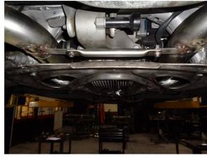
**Step 3.** Next slip the inlet of both Mid Pipes over the outlets of the Resonator Assembly and loosely secure using the supplied clamps, loosely install the brace using the OE fasteners Install the two Tail Pipe Assemblies in a similar fashion. Locate the welded hangers to the rubber insulators.
