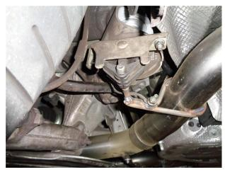
**Step 4.** Complete the installation by attaching the Muffler Assemblies to the Mid Pipes using the supplied 3.00" clamps. Fit the hangers on the Muffler Assemblies into the rubber insulators and reattach the factory braces and covers. Re-attach the ground straps to the mufflers.
