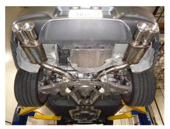
**Step 5.** Once a final position has been chosen for the new system, evenly tighten all clamps from front to rear using the torque specifications on page one of the instructions. Inspect all fasteners after 25-50 miles of operation and re-tighten if necessary.
