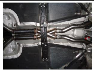
**Step 2.** To install your new MAGNAFLOW exhaust system the Inlet Pipe Assemblies need to be assembled loosely with the Resonator Assembly using the supplied clamps first. Install the completed assembly by attaching the inlet flanges to the catalytic converter outlets using the OEM hardware. Locate the four mounting brackets to the vehicle sub frame using the supplied hardware
