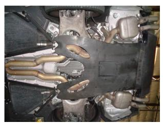
**Step 1.** To remove the OEM exhaust system begin by removing the frame cross brace, the exhaust brace and cover at the rear of the vehicle. Also unfasten the groud strap located on both muffler assemblies. Next unbolt the inlet pipe flanges at the catalytic converters. Working front to rear with the exhauset supported disengage or unfasten all hangers and remove the exhaust. Retain all hardware and insulators as they will be use to install the new system.
