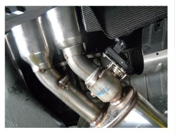
Step 6: Re-connect the wiring harness plugs to the Valve motors.
