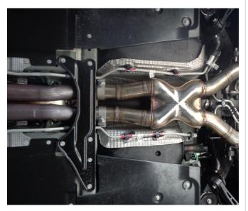
Step 4: Begin installation of the new system by sliding the X-Pipe Assembly inlets onto the cut outlets of the OEM exhaust and loosely fasten with the supplied 2.75" clamps. (at this time slide the loose end of the cut heatshield under the clamps before tightening). Fit hangers into rubber insulators.
