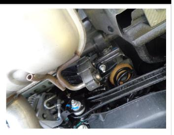
Step 3: Working front to rear disengage all welded hangers from the rubber insulators and remove the system. (Retain the insulators as they will be needed to mount the new MAGNAFLOW system.) Once the OEM system is on the ground transfer the valve motors over to the new Magnaflow exhaust system.
