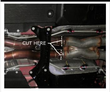
Step 1: It is necessary to cut the factory exhaust system to install the new Magnaflow unit. To do this cut the band clamps holding the heat shield to the pipes in front of the X. Move the heatshield out of the way and cut 1.5" in front of the welds on the factory X-Pipe. Deburr the cut pipes to facilitate installation of the new system.
