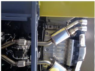
Step 5: Install the Muffler Assemblies to the X-Pipe Assembly with the supplied 3.00" clamps and engage the welded hangers to the rubber insulators. Leave all clamps loose for final adjustment of the system.
