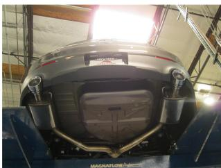
**Step 3.** Next attach the Y-Pipe Assembly to the Resonator Assembly and then the Muffler Assemblies to the Y-Pipe using the supplied 2.50" clamps. Insert hangers into rubber insulators.
