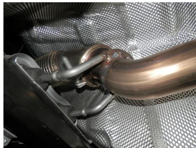
**Step 4.** Begin installation of the MagnaFlow exhaust by attaching the Inlet Pipe Assembly to the flex outlet using the factory clamp and fitting the hangers into the rubber insulators.
