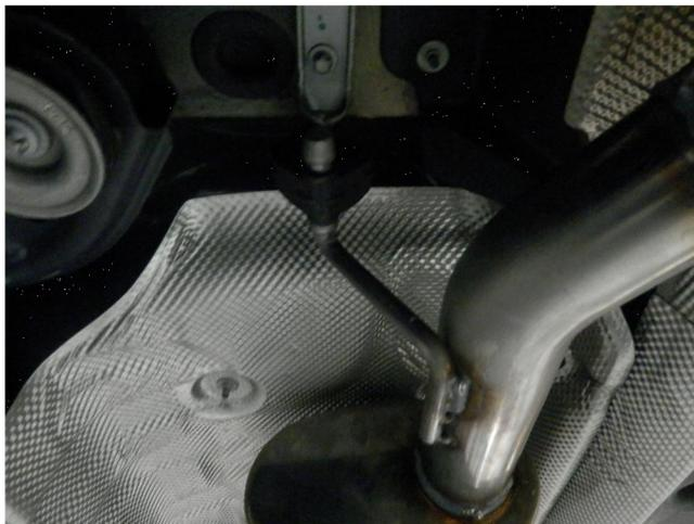
**Step 6.** Complete installation by attaching the Muffler Assembly to the Mid-Pipe using a supplied 2.50" clamp and fitting the hangers into the rubber insulators. Re-attach cross braces.
