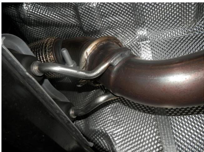
**Step 2.** Begin removing the OEM exhaust by unfastening the clamp located behind the flex pipe.
