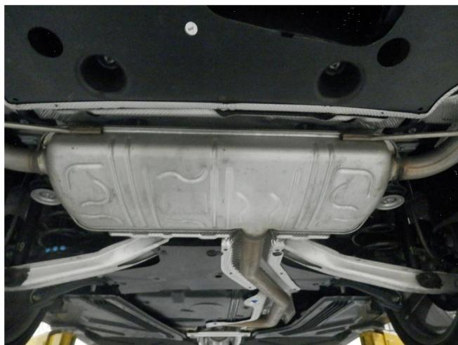
**Step 3.** With the exhaust supported, work front to rear and extract the welded hangers from the rubber insulators. Do not discard or damage the clamp or insulators as they will be re-used to install the new MagnaFlow exhaust.
