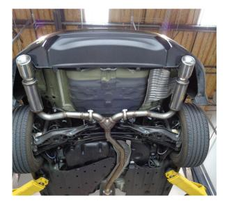
**Step 6.** Loosely attach both driver and passenger side Muffler Assembly flanges to the Y-Pipe Assembly. Secure with the supplied gaskets and hardware. Engage welded hangers to rubber isolators.
