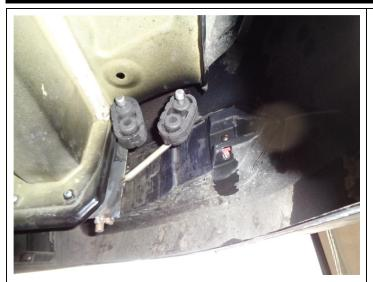
**Step 5.** Using the supplied hardware and rubber hangers, bolt the new bracket to the driver side.
