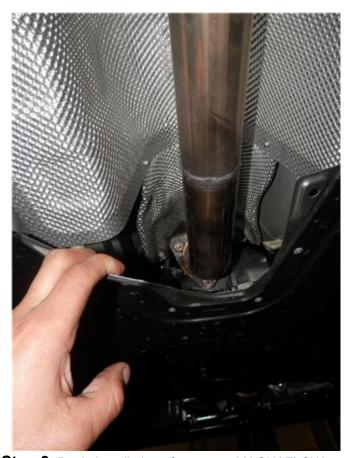
**Step 3.** Begin installation of your new MAGNAFLOW system by attaching the Inlet flange of the Inlet Resonator Assembly to the catalytic converter outlet using the OEM fasteners. Engage the welded hanger to the rubber isolator. Keep all fasteners and clamps loose until final adjustment.
