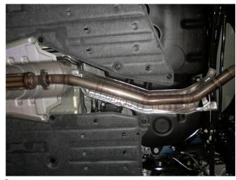
**Step 4.** Next attach the Y-Pipe Assembly to the Inlet Resonator Assembly by coupling the flanges using the supplied gasket and hardware.
