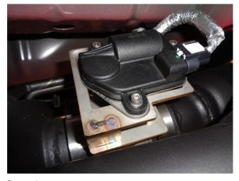
**Step 6**. If your vehicle has valves, re-connect the wiring harness plugs to the Valve motors and wire mounting bracket. If not yet purchased, Valve Kit is part# 10805
