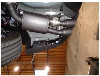
**Step 5.** Finish the initial installation by fitting the Muffler Assemblies onto the Mid pipe Assemblies using the supplied 3.00" clamps and inserting the hangers into the rubber insulators.
