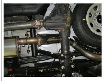
**Step 4.** Next install the over axle Resonator assembly to the Muffler in the similar fashion using the supplied 3.50" clamp, fitting the welded hangers into the rubber insulators.
