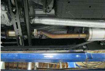
**Step 1.** To remove the OEM exhaust system, you will to need to cut the pipe behind the muffler before it goes over the axle. Disengage the welded hangers from the rubber insulators and remove the tailpipe. Next remove the fasteners from the two bolt fange behind the catlytic converter. Do not damage or discard the fasteners or rubber insulators, as they will be re-used to mount the new system. Disengage the remainder of the hangers and remove the system.
