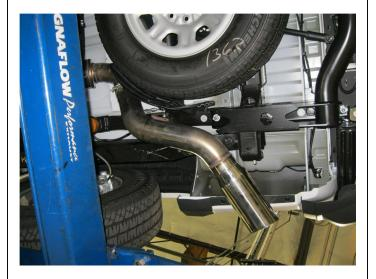
**Step 5.** Finish by installing the Tail Pipe Assembly to the over axle Resonator assembly using the supplied 4.00" clamp, fitting the welded hanger into the rubber insulator.
