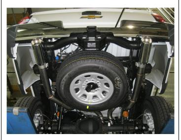
**Step 5.** Finish by installing the Tail Pipe Assemblies to the over axle Extension Pipe Assemblies and the Tips to the Tail Pipe Assemblies using the supplied 3.00" clamps and fitting the welded hangers into rubber insulators. Use the two Ø3.00x7.00" Extension Pipes between the Tail Pipe Assemblies and the Tips if your truck has a Long Bed configuration.
