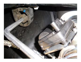
Step 6: If your vehicle has valves re-connect the wiring harness plugs to the Valve motors, re-install the rear valance.
