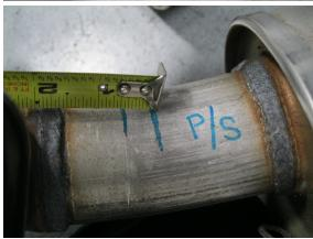
Step 3: Begin removing the OEM exhaust system by cutting both pipes going into the muffler assemblies. Measure and cut 2.0" driver side, 1.75" Passenger side, behind the exhaust valve welds as shown. Next extract the hangers from the rubber insulators and remove the OEM mufflers. Retain rubber insulators and as they will be used to install the new system
