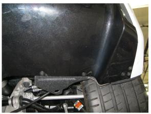
**Step 1.** To remove the OEM exhaust system you will first need to remove the rear valance. To do so you will need to remove The two 10mm bolts behind each reflector, the two 10mm bolts behind the license plate and two more 10mm bolts just underneath the license plate. Then you will need to remove the five 8mm bolts on both sides of the valance underside and remove it.
