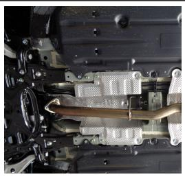
**Step 2:** Begin installing your new system by loosely bolting both inlet flange of the Inlet Assemblies to the catalytic converter outlets using the OEM hardware. Engage the welded hangers to the rubber insulator.
