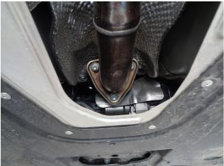
**Step 1:** To remove the OEM system first unbolt and remove the cross member at the inlet. Next, unbolt the inlet pipe at the catalytic converter flange junctions. Working front to rear disengage all welded hangers from the rubber insulators. The OEM exhaust system can now be removed in one piece. Be sure to retain all mounting hardware as it will be needed to install your new MAGNAFLOW system
