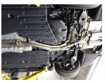
**Step 3:** Next loosely fasten the Mid Extension Pipe to the Resonator Assembly using the supplied clamp.
