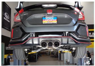
**Step 5:** Once a final position has been chosen for the new exhaust system, evenly tighten all clamps from front to rear using the torque specifications on page one of these instructions. Inspect all fasteners after 25-50 miles for operation and re-tighten if necessary.
