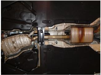
Step 1: To remove the OE system you will need to remove the cross brace located between the underbody resonators and the two braces located near the rear mufflers. Begin by loosening the band clamp attaching the exhaust between the OE resonators. Working front to rear disengage all welded hangers from the rubber insulators. The OE exhaust system can now be removed in one piece. Be sure to retain all mounting hardware as it will be needed to install your new MAGNAFLOW system
