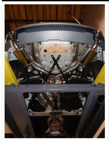
Step 4: Finish by attaching the driver and passenger side Muffler Assemblies to the Y-Pipe Assembly using the supplied 2.50" clamps and engaging the hangers to the rubber insulators. Reattach all braces.
