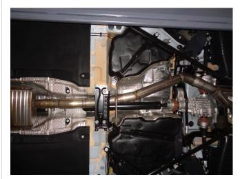
Step 2: Begin installing your new system by loosely attaching the Inlet Pipe Assembly by inserting it into the OE band clamp. Engage both hangers to the rubber insulators.
