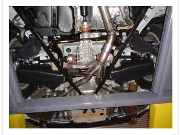
Step 3: Next fasten the Y-Pipe Assembly to the Inlet Assembly using the supplied 3.00" clamp.
