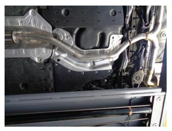
Step 4: Next use the supplied 2.250" clamp to attach the Y-Pipe Assembly to the Resonator Assembly and insert the hanger to rubber insulator.
