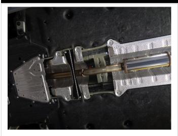
**Step 3.** Begin installation of your new MAGNAFLOW system by attaching the Resonator Assembly to the catalytic converter outlet using the OEM fasteners and insulator and the supplied ring gasket. Keep all fasteners and clamps loose until final adjustment.
