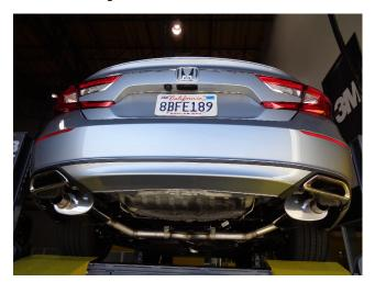
Step 6: Once a final position has been chosen for the new exhaust system, evenly tighten all clamps from front to rear using the torque specifications on page one of the instructions and re-install OE braces. Inspect all fasteners after 25-50 miles of operation and re-tighten if necessary.
