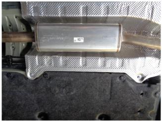
Step 2: Next unfasten the front 3 bolt flange located behind the catalytic converter, extract the hangers from the rubber insulators and remove the remaining part of the OE system.
