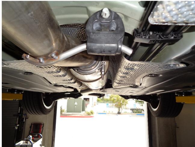
Step 2: Begin installing the new system by attaching the Inlet Assembly flange to the catalytic converter outlet using the OEM hardware. Engage the welded hanger to the rubber insulator. Keep all clamps and fasteners loose until final adjustment
