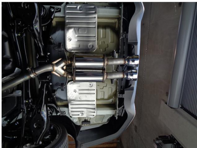
Step 4: Finish by loosely installing the Muffler Assembly to the Mid Extension pipe using the supplied clamp and fitting the hangers into the rubber insulators.
